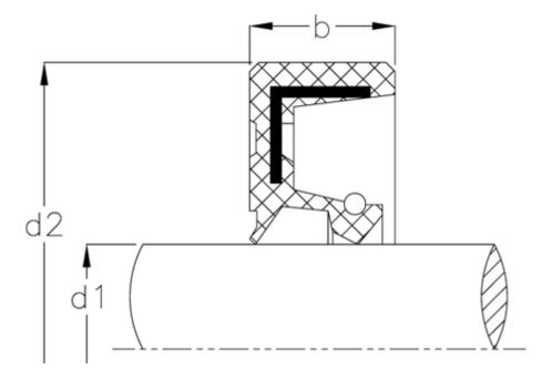
$\begin{array}{ll} b & = 7 \\ d1 & = 30 \\ d2 & = 50 \\ Material = NBR \end{array}$
